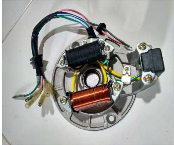
Gambar 4.21 Bentuk spul pengapian (source coil ignition)
