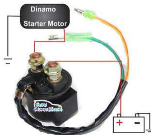
Gambar 2.53 Pengujian relay starter
